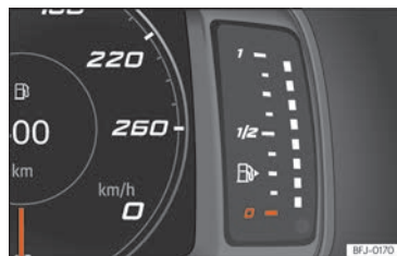
Billede 6 Kombiinstrument SEAT Digital Cockpit: tankmåler
