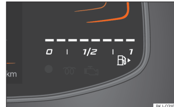
Billede 5 Kombiinstrument Basic: tankmåler
