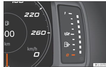
Billede 6 Kombiinstrument SEAT Digital Cockpit: tankmåler
