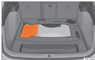
Billede 235 Plug-in-hybridbiler (PHEV): batteriets placering i bagagerummet
