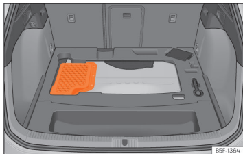
Billede 229 Plug-in-hybridbiler (PHEV): batteriets placering i bagagerummet
