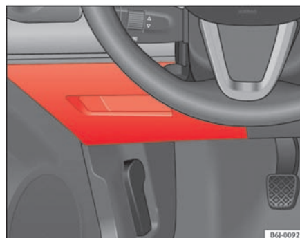
Fig. 127 Sikringer i instrumentpanelet
