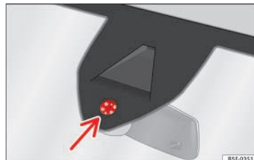
Fig. 143 Regnsensorens sensitive flade
