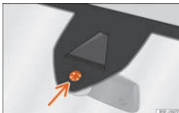
Fig. 157 Regnsensorens sensitive flade
